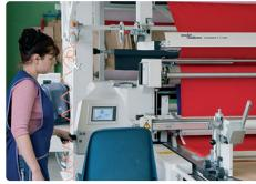
Operator of a highly automated cloth-cutting and spreading complex at work
