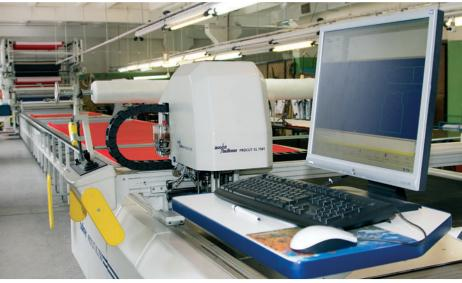
Automatic cloth-cutting and spreading complex Bullmer at Viazma clothing factory
